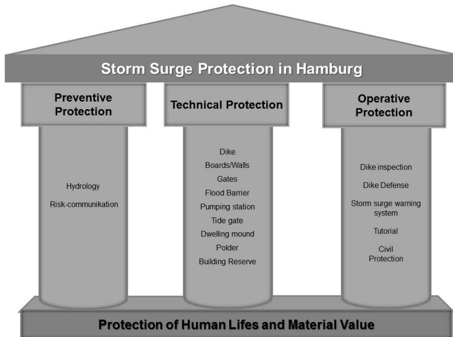
Fig. 2: Structure of Coastal Protection in Hamburg (Free and Hanseatic City of Hamburg, LSBG)
